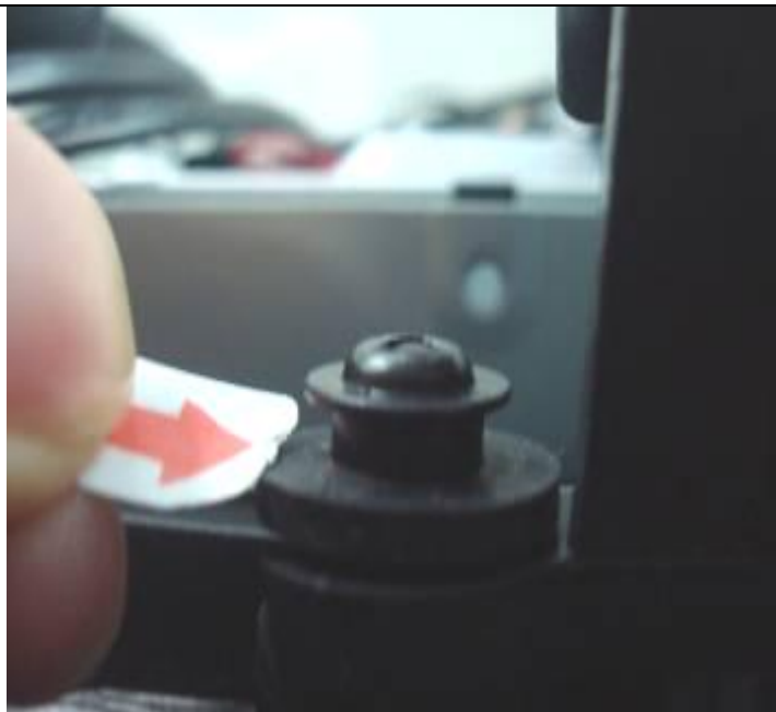
3.1.2 Internal check 3pcs, found right Speaker fixing too loose because screw pole too long, at present when listen to music the speaker not shake to noise, but if clients long time to use maybe lead to shake to noise, advise to improve this problem
